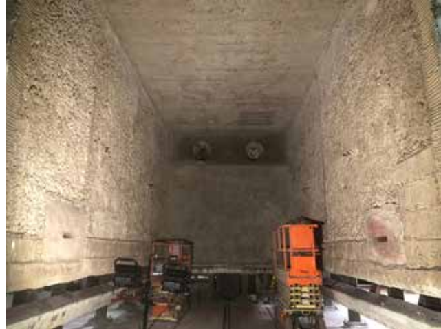
Fully coated forge furnace with ITC 100HT ceramic lining
