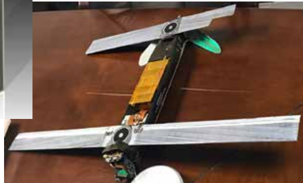
U.S. Army's UAV which uses high-power form-factored Li/CFx battery
