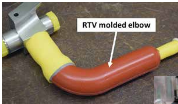
ABOVE: Representative transfer line assembly produced without using AM
